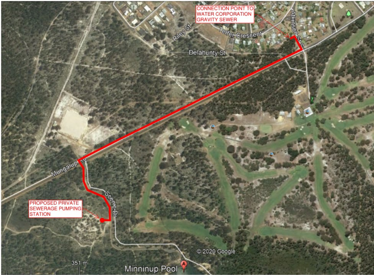
Figure 5 Proposed sewer Pressure Main Alignment
