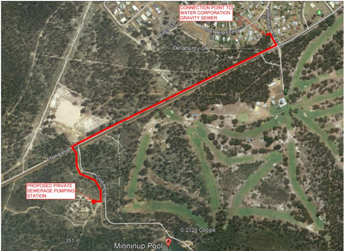
Figure 7 Proposed sewer Pressure Main Alignment
