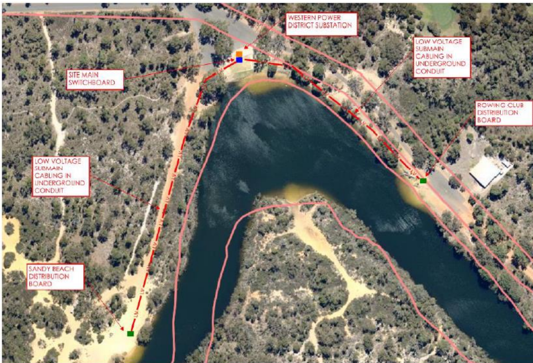
Figure 25: Minningup Pool Main Electrical Components Reference River Engineering
