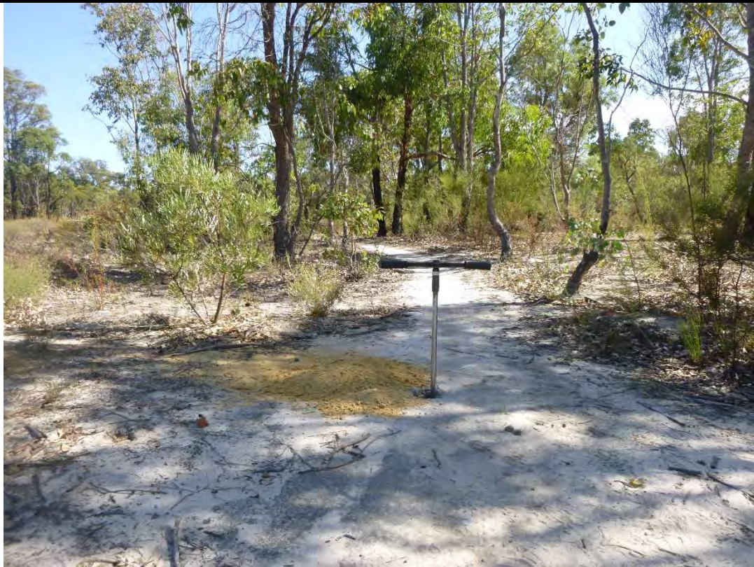
Photo 7. Test Location 02 (TH02), Sub-surface probing by using a hand auger
