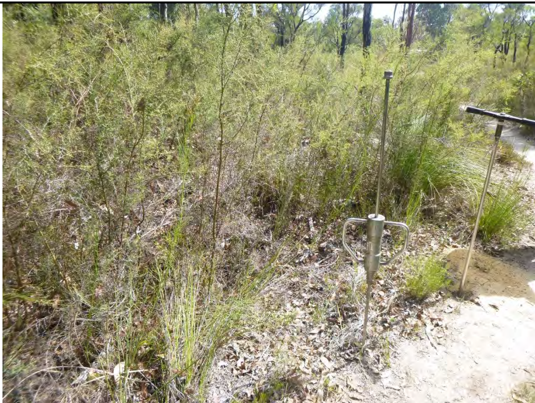
Photo 26. Test Location 18 (DCP18), Testing by a Dynamic Cone Penetrometer
