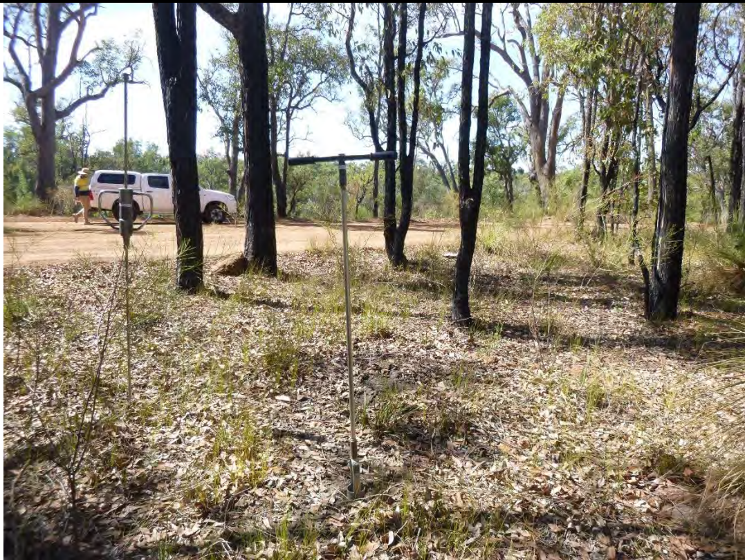
Photo 35. Test Location 26 (TH26), Sub-surface probing by using a hand auger
