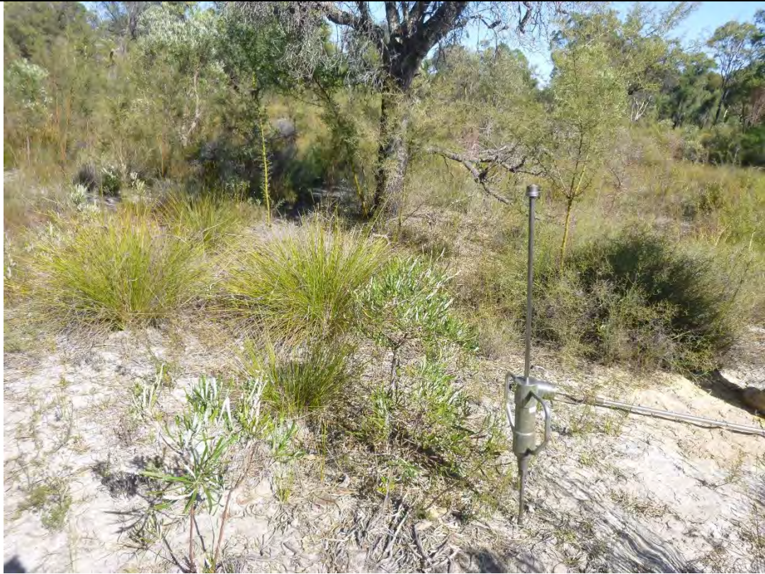
Photo 19. Test Location 14 (DCP14), Testing by a Dynamic Cone Penetrometer
