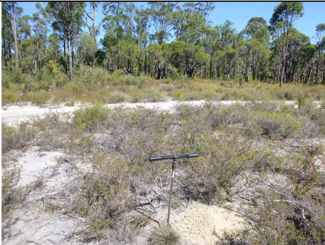
Photo 9. Test Location 04 (TH04), Sub-surface probing by using a hand auger
