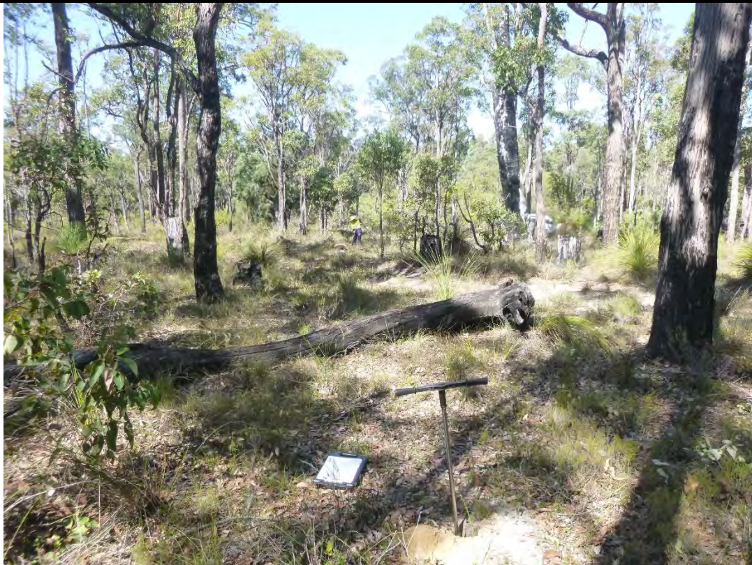
Photo 31. Test Location 23 (TH23), Sub-surface probing by using a hand auger
