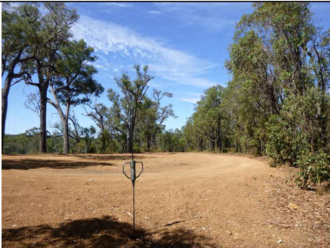
Photo 34. Test Location 25 (DCP25), Testing by a Dynamic Cone Penetrometer
