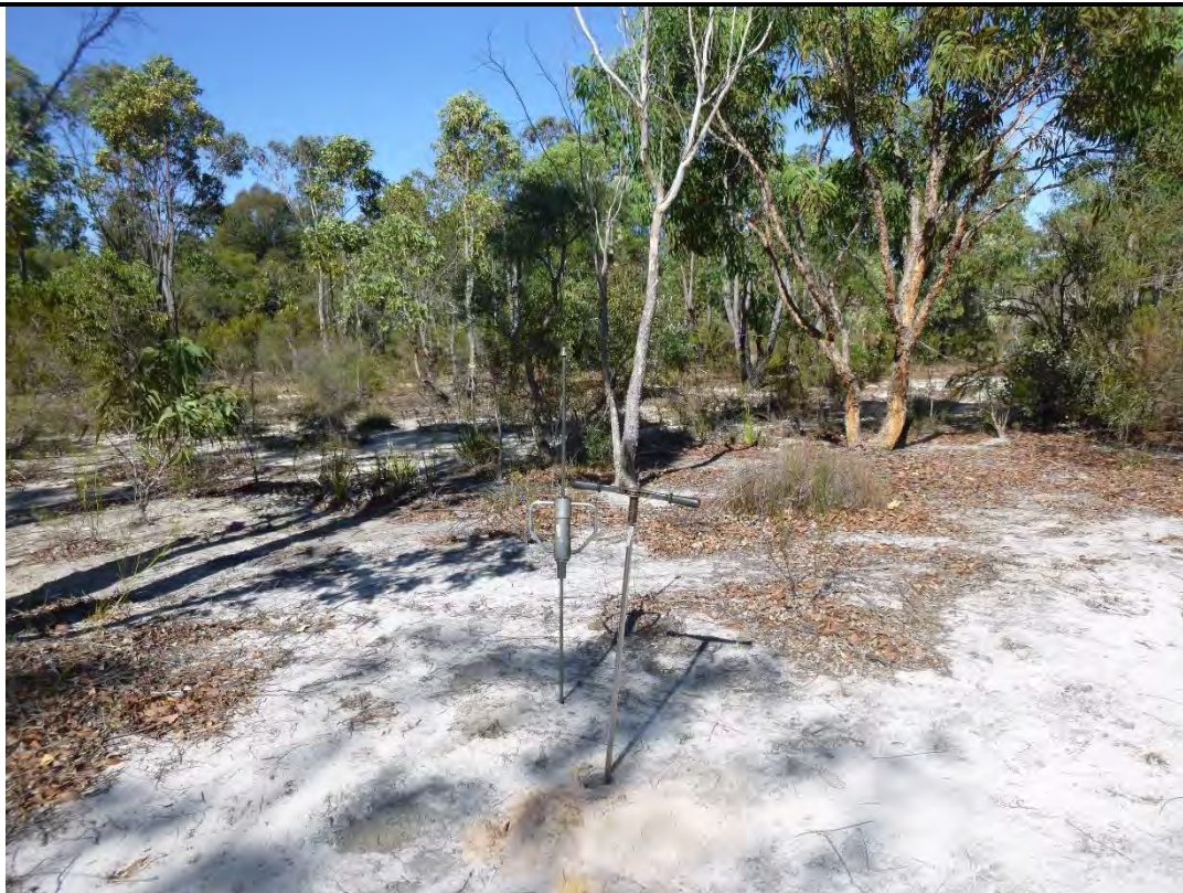
Photo 15. Test Location 10 (TH10), Sub-surface probing by using a hand auger
