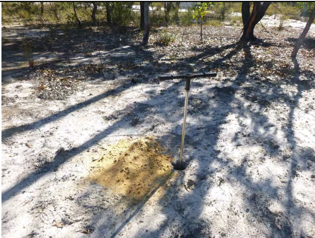
Photo 14. Test Location 09 (TH09), Sub-surface probing by using a hand auger
