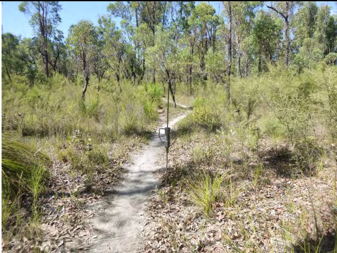
Photo 27. Test Location 19 (DCP19), Testing by a Dynamic Cone Penetrometer
