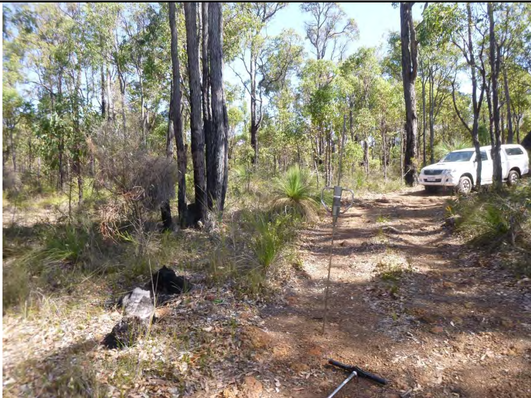
Photo 38. Test Location 29 (DCP29), Testing by a Dynamic Cone Penetrometer
