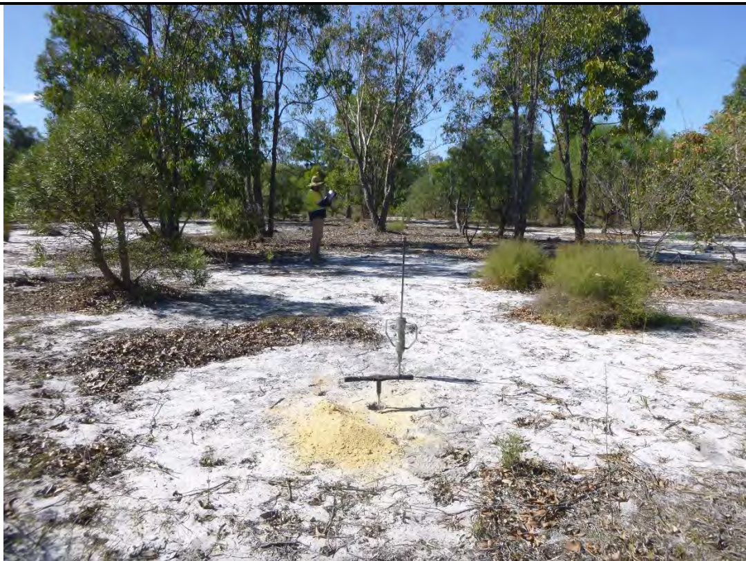
Photo 18. Test Location 13 (TH13), Sub-surface probing by using a hand auger
