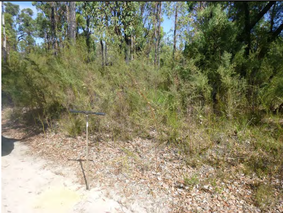
Photo 22. Test Location 16 (TH16), Sub-surface probing by using a hand auger
