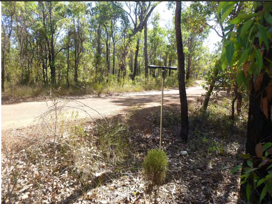
Photo 40. Test Location 30 (TH30), Sub-surface probing by using a hand auger
