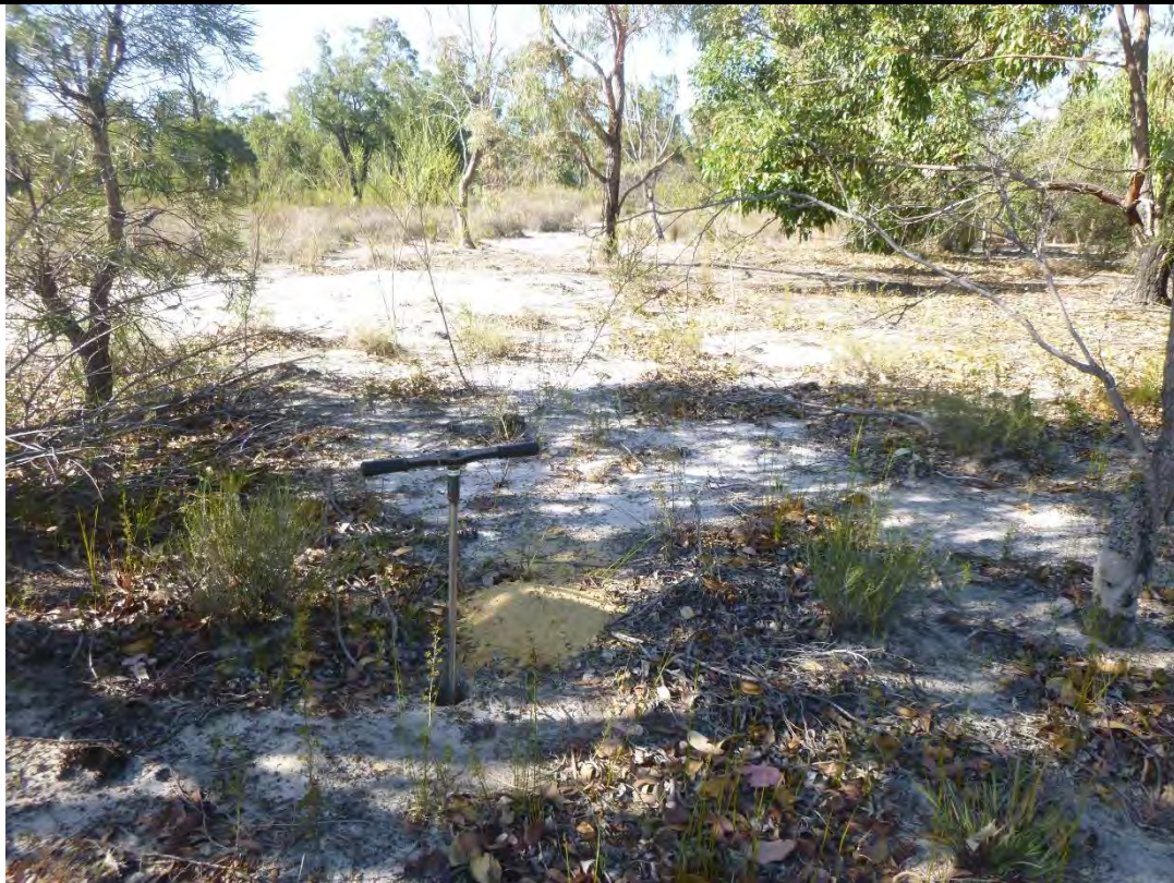
Photo 13. Test Location 08 (TH08), Sub-surface probing by using a hand auger
