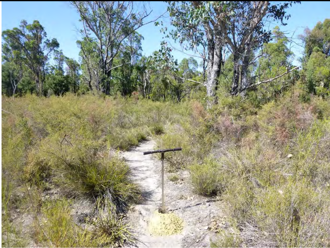
Photo 5. Test Location 01 (TH01), Sub-surface probing by using a hand auger
