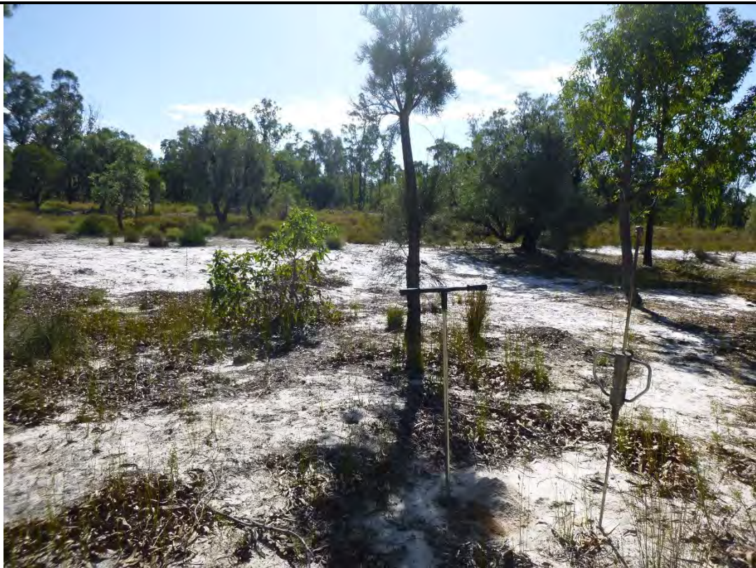
Photo 17. Test Location 12 (TH12), Sub-surface probing by using a hand auger
