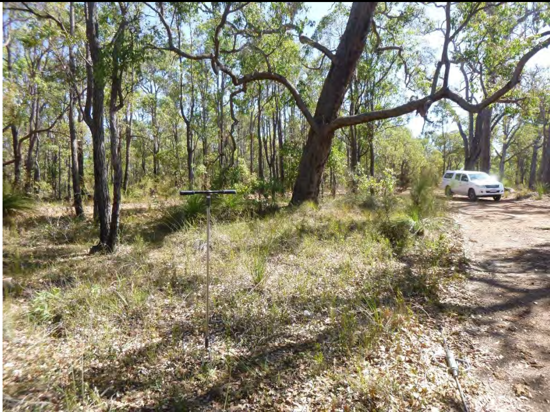
Photo 37. Test Location 28 (TH28), Sub-surface probing by using a hand auger
