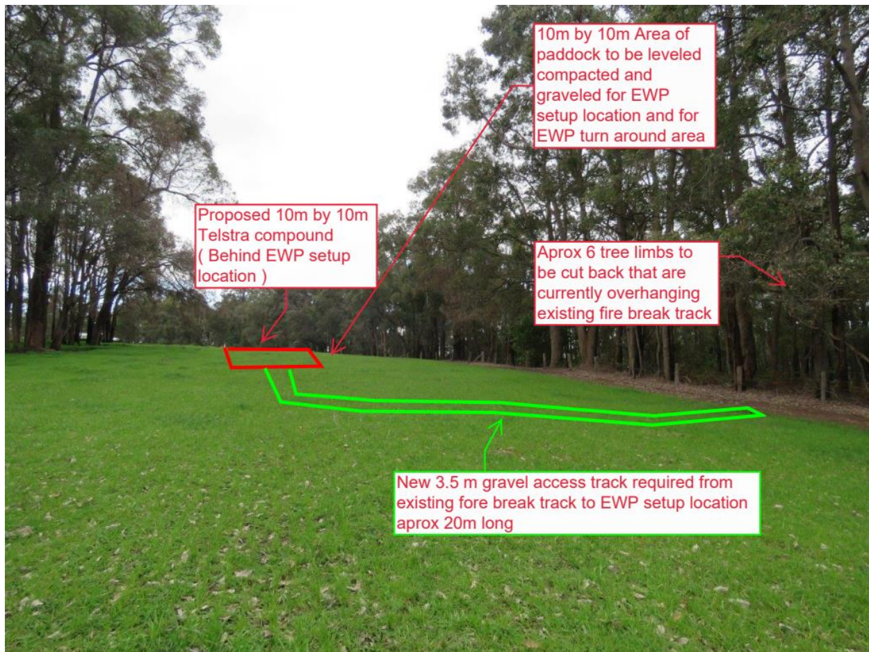
Figure 12 Space for temporary crane and works setup near the proposed 10m x 10m Amplitel compound Source: Ventia 2022
