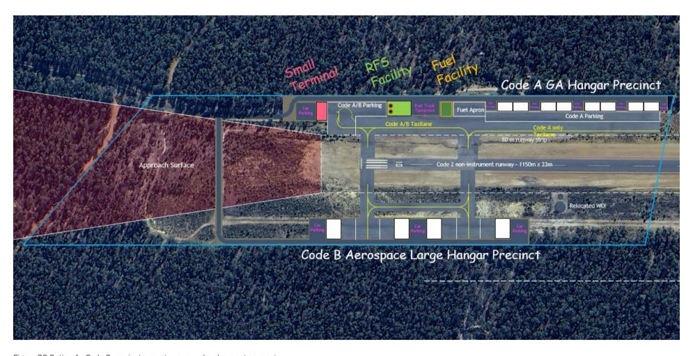
Figure 30 Option 1 - Code 2 non-instrument runway - development concept
