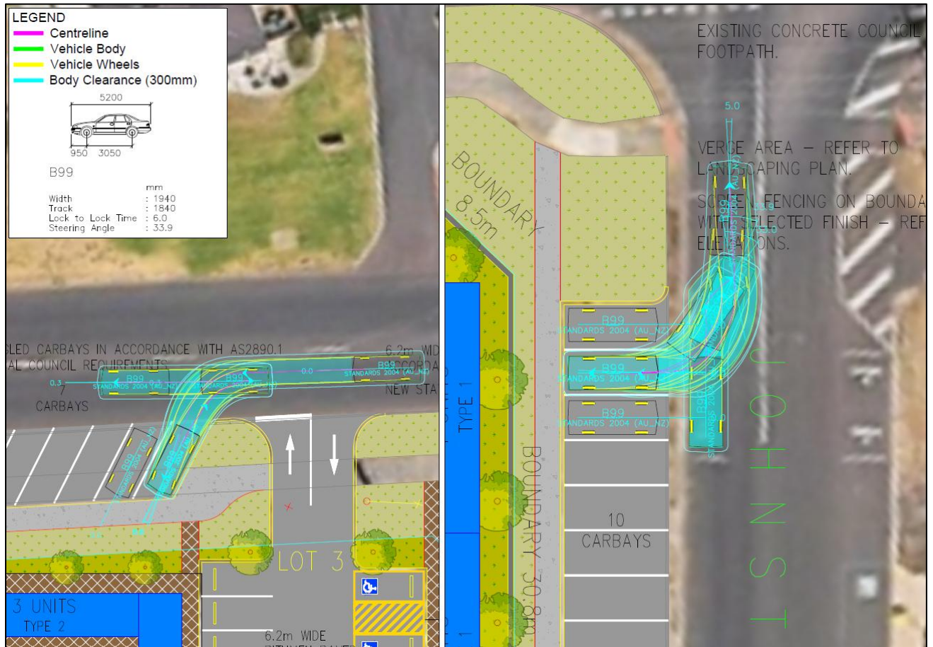
Figure 12 B99 On-street Parking
